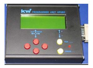
The Hand-held Programming Unit HPG-60 is the universal programming tool for the entire control system. It is equipped with 6 keys, a four-lined LCD-display, one red LED, and a 9-pole RS232-Interface. Through the HPG-60, all parameters can be displayed and changed. Current actions of the control system are displayed though permanent status indicators. The accumulated fault events can be read out from the fault memory. Inquiries can also be initiated through this unit.
