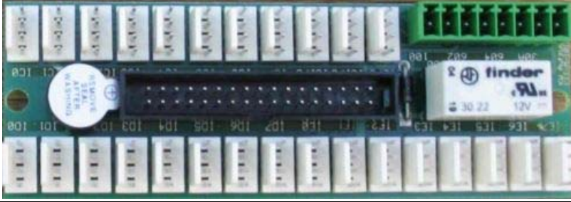
CAR PANEL PCB EIT-2005 MOLEX, with molex plugs for push buttons of KW 40,44, 46 und 60:
